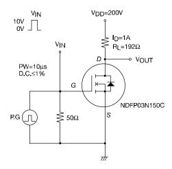
Fig.3 Reverse Recovery Time Test Circuit
