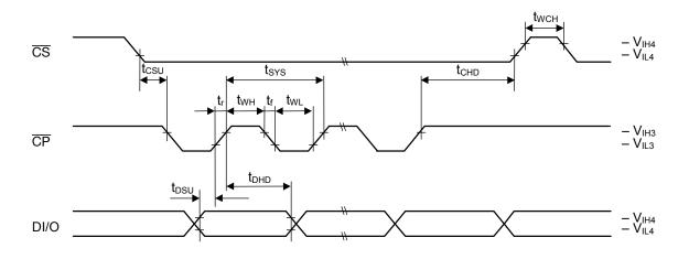
Clock synchronous serial interface input/output timing
