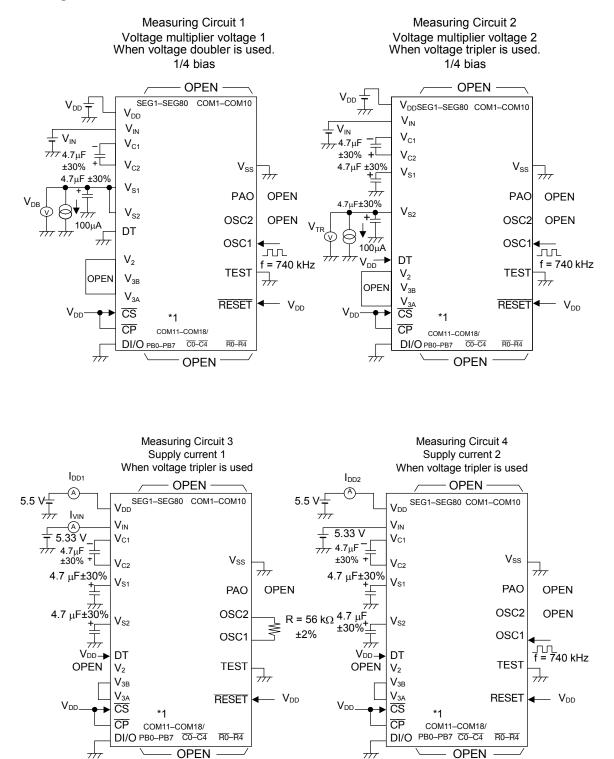
\*1: PB0 - PB7 for ML9090A-01, and COM11 - COM18 for ML9090A-02
