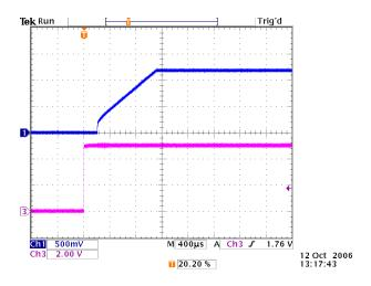
Load transient, 0 - 3A,  $V_{IN}/V_{OUT} = 5.5V/3.3V$
