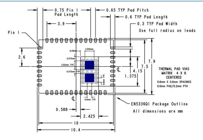
Figure 6: EN5336QI PCB Footprint (Top View)
