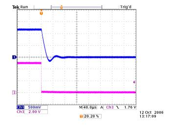
Start-up waveform,  $V_{IN}/V_{OUT} = 5.5V/1.2V$
