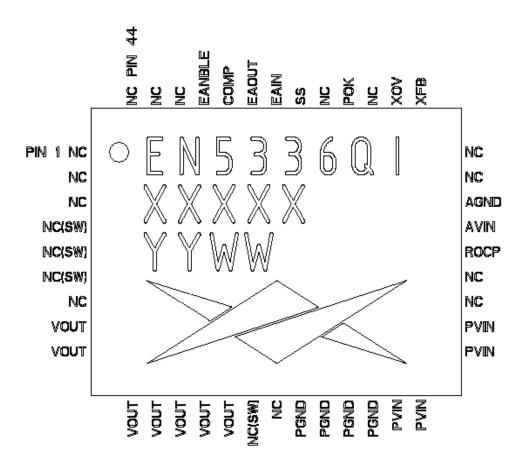
Figure 2. Pin-out diagram, top view.
