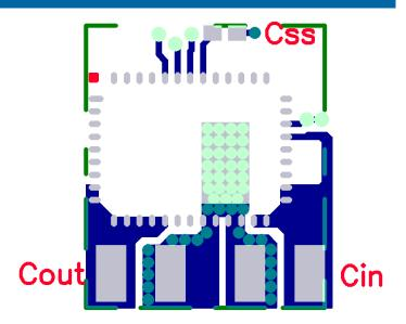
Figure 4: Top PCB Layer Critical Components and Copper for Minimum Footprint
