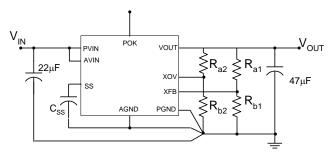
**Figure 4.** V<sub>OUT</sub> and OVP resistor divider networks.
