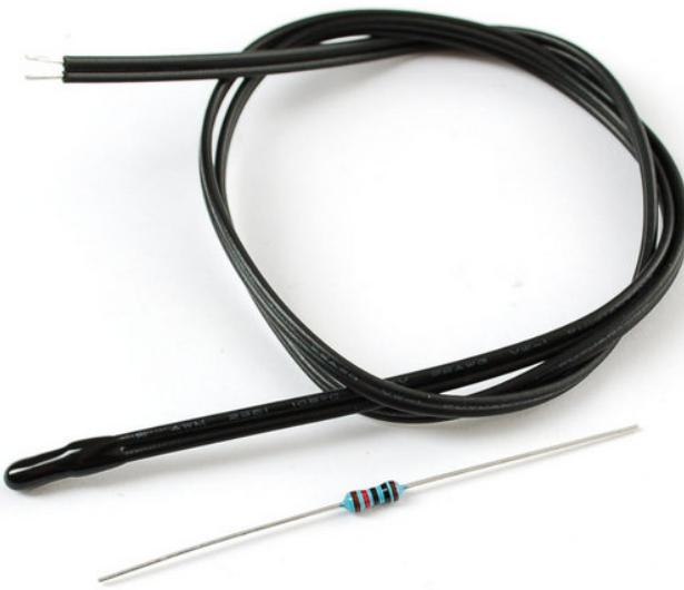
There are two kinds of of thermistors, NTC (negative temperature coefficient) and PTC (positive temperature coefficient). In general, you will see NTC sensors used for temperature measurement. PTC's are often used as resettable fuses - an increase in temperature increases the resistance which means that as more current passes thru them, they heat up and 'choke back' the current, quite handy for protecting circuits!
