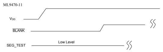
\* After  $V_{DD}$  is applied,  $\overline{BLANK}$  and  $SEG\_TEST$  should be applied to 'L' level to make all SEGMENTS off until first group of display data is latched.
