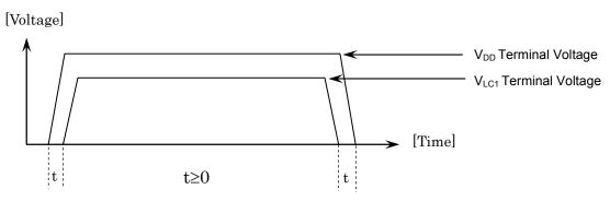
\*  $V_{\text{LC1}}$  and  $V_{\text{LC2}}$  are applied when  $V_{\text{DD}}$  is applied to external bias resistor.
