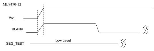
\* When VDD is applied, BLANK should be applied to 'H' level at the same time, and SEG\_TEST should be applied to 'L' level to make all SEGMENTS off until first group of display data is latched.
