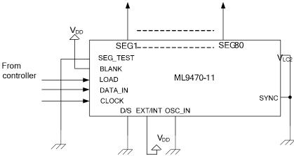
\*The output logic can be reversed with respect to the input data by setting OSC\_IN to "H" level.
