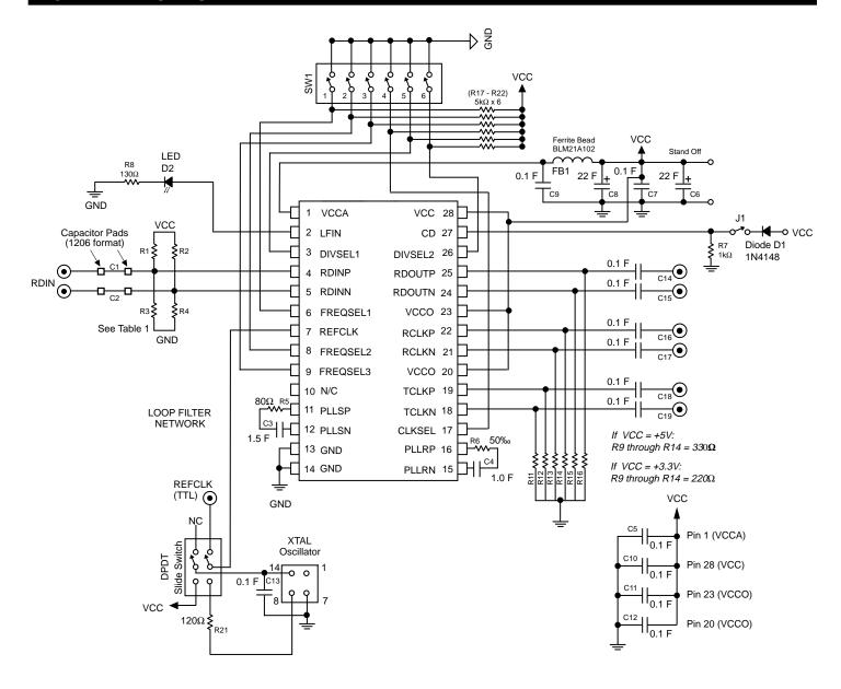
Note 1. C5 and C10–C12 are decoupling capacitors and should be kept as close to the power pins as possible.
