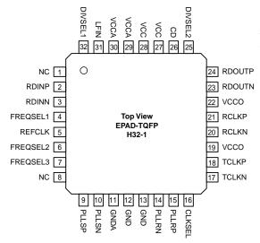
32-Pin EPAD TQFP (H32-1)
