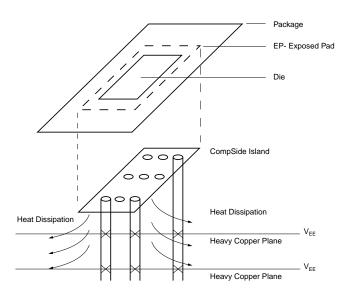
PCB Thermal Consideration for 32-Pin EPAD-TQFP Package
