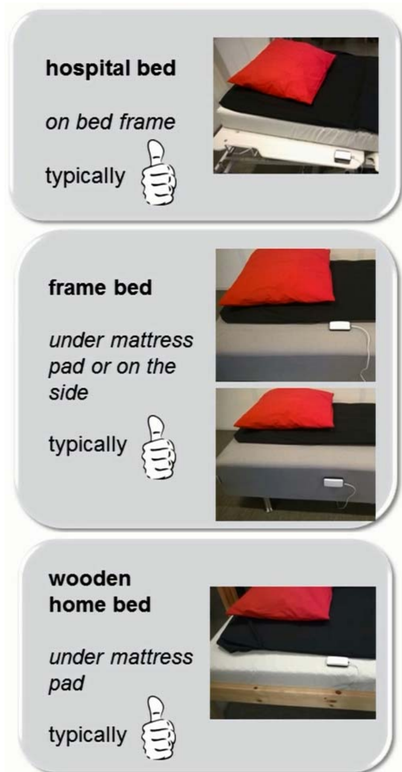
Figure 5. Examples of good SCA11H attachment positions
