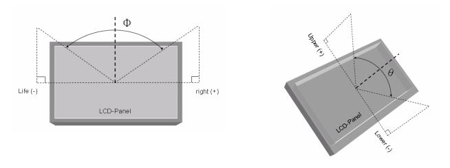
Fig.3 Definition of Viewing Angle
