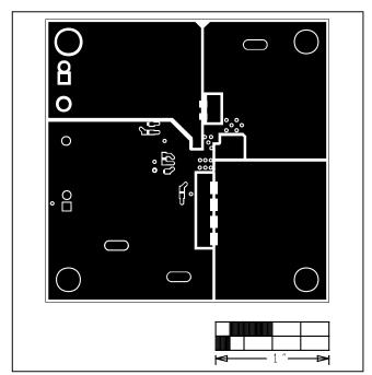
Figure 6. MAXM17504 EV Kit PCB Layout—Solder Side
