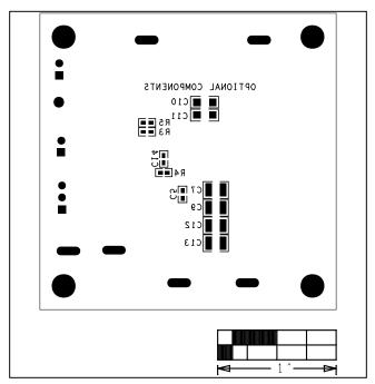
Figure 2. MAXM17504 EV Kit Component Placement Guide—Solder Side
