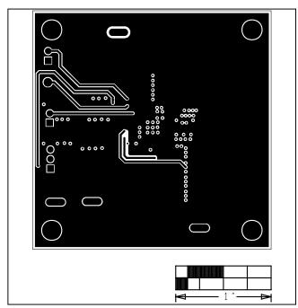
Figure 5. MAXM17504 EV Kit PCB Layout—PGND Layer 3
