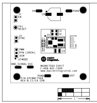
Figure 1. MAXM17504 EV Kit Component Placement Guide—Component Side
