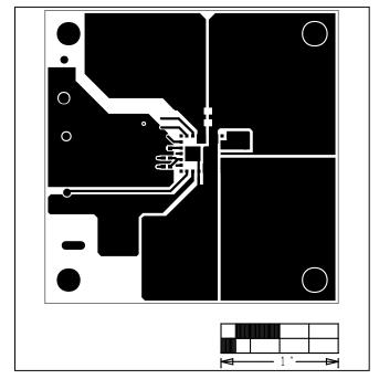
Figure 3. MAXM17504 EV Kit PCB Layout—Component Side
