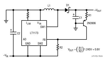
Figure 8. Negative-to-Positive Converter
