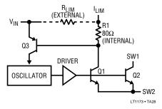
Figure 11. LT1173 Current Limit Circuitry
