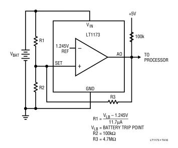
Figure 12. Setting Low Battery Detector Trip Point
