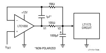
Figure 1. Test Circuit Measures No Load Quiescent Current of LT1073 Converter
