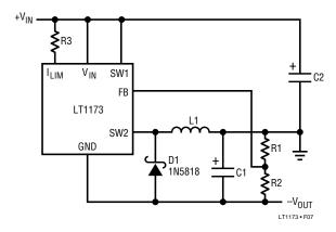
Figure 7. Positive-to-Negative Converter
