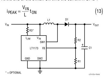
Figure 5. Step-Up Mode Hookup. Refer to Table 1 for Component Values
