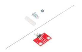
**Description:** These simple switches are the Mechanical Bumper sensor for the SparkFun RedBot, giving you the ability to detect a collision before it really happens. This sensor works by acting as a SPST switch. When the "whisker" bumps into a foreign object it will make contact with a nut next to it, closing the connection and, by default, turning off the motor. By attaching these mechanical bumpers to you robot the whisker will bump something before your robot crashes into it.
