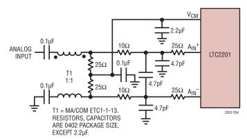
Figure 4. Using a Transmission Line Balun Transformer.
