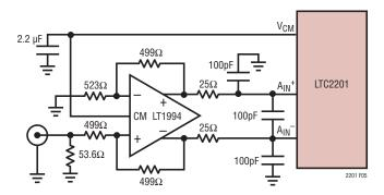
Figure 5. DC Coupled Input with Differential Amplifier
