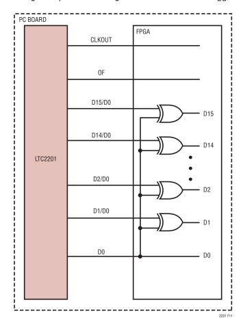
Figure 11. Descrambling a Scrambled Digital Output
