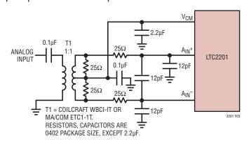
Figure 3. Single-Ended to Differential Conversion Using a Transformer. Recommended for Input Frequencies from 1MHz to 100MHz
