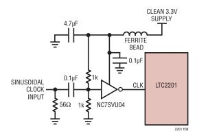
Figure 8. Sinusoidal Single-Ended CLK Drive
