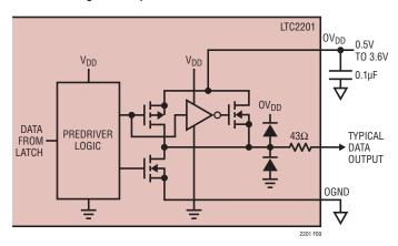
Figure 9. Equivalent Circuit for a Digital Output Buffer
