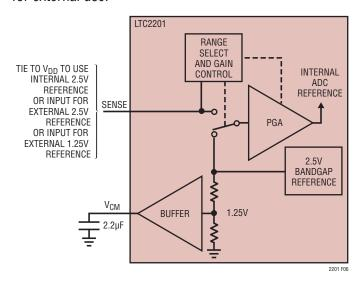
Figure 6. Reference Circuit
