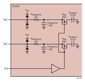
Figure 2. Equivalent Input Circuit
