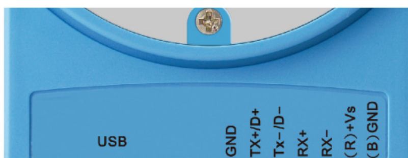
Figure 1.9 RS-422/485 and USB interface of ADAM-2520Z.
