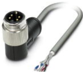
Bus system cable, DeviceNet, 5-position, PUR halogen-free, Gray RAL 7001, Plug angled 7/8"-16UNF, on Free cable end, Cable length: 15 m
