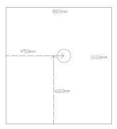
Test Baffle (speaker mounted in circle)
