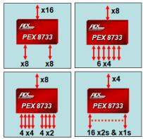
Figure 1. Single-Host Port Configurations
