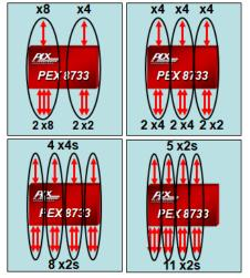
Figure 2. Multi-Host Port Configurations
