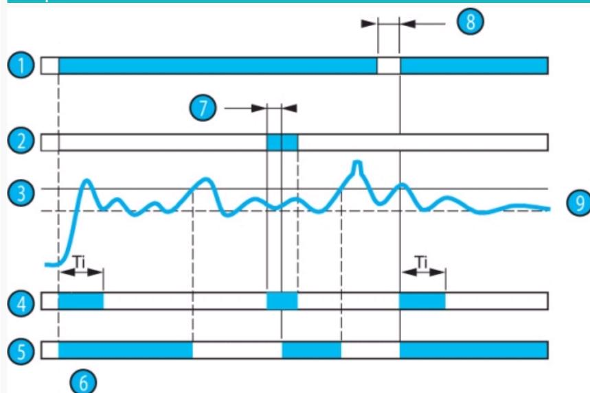
When the HSV has been configured in "memory" mode, if overspeed is detected, the output relay stays in the rest state ("alarm") irrespective of any subsequent change in the speed of the process. It will not be able to revert to ("normal") operating state until contact S2 closes (50 ms minimum). If, when S2 reopens, the speed is too high, the relay reverts to the rest latched state ("alarm").
