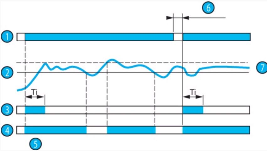
After the end of the inhibit delay on starting, "TI", as soon as the measured speed drops below the threshold value, the output relay changes state, from operating point to rest position ("alarm" operational state, 11-14 open and 11-12 closed).
