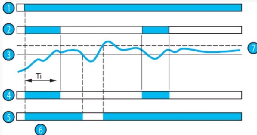
On energisation, to allow the controlled process to reach its nominal operating speed, the HSV relay is inhibited for a period that is adjustable from 0.6 to 60 seconds.
