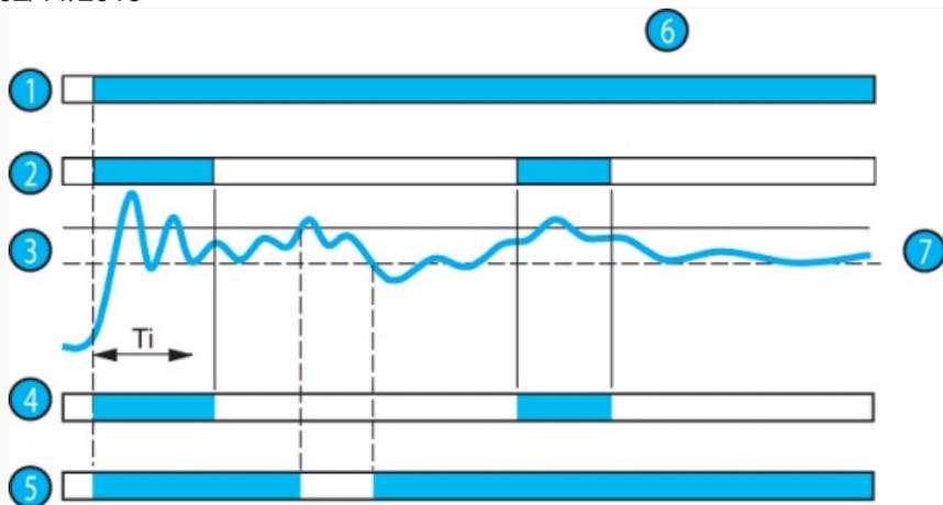
It is possible to inhibit the HSV relay by closing external contact S2 until the process has reached its nominal speed.
