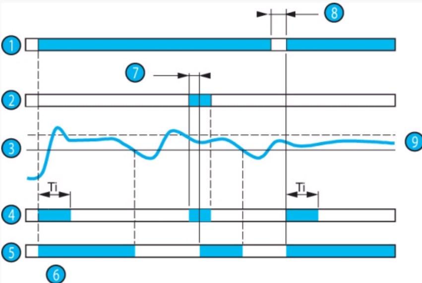
When the HSV has been configured in "memory" mode, if underspeed is detected, the output relay stays in the rest state ("alarm") irrespective of any subsequent change in the speed of the process.
