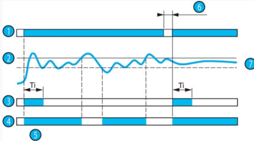
After the end of the inhibit delay on starting, "Ti", as soon as the measured speed rises above the threshold value, the output relay changes state, from operating point to rest position ("alarm" operational state, 11-14 open and 11-12 closed).
