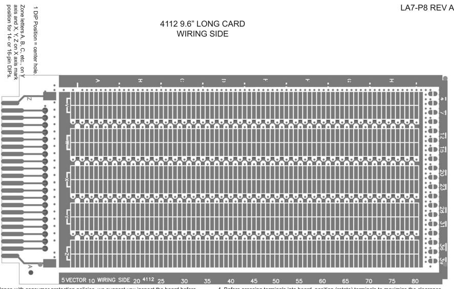
5. In accordance with consumer protection policies, we suggest you inspect the board before assembly to verify adequate clearance will exist between the ground plane surrounding the holes and any leads or terminals installed in holes so that shorting will not occur. Terminals inserted into the holes in the ground plane areas, and closely spaced contact finger areas may cause short circuits unless:
