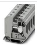
Feed-through terminal block, with Allen screws, Connection method: Screw connection, Cross section: 1.5 mm<sup>2</sup> - 50 mm<sup>2</sup>, AWG: 16 - 1/0, Width: 16 mm, Color: gray, Mounting type: NS 35/7,5, NS 35/15
