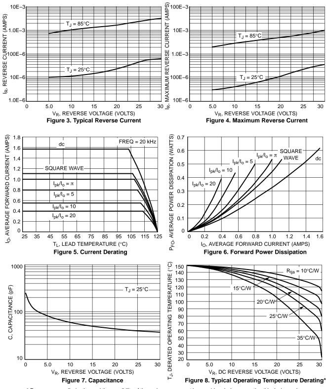
\* Reverse power dissipation and the possibility of thermal runaway must be considered when operating this device under any reverse voltage conditions. Calculations of T<sub>J</sub> therefore must include forward and reverse power effects. The allowable operating T<sub>J</sub> may be calculated from the equation:  $T_J = T_{Jmax} - r(t)(Pf + Pr)$  where
