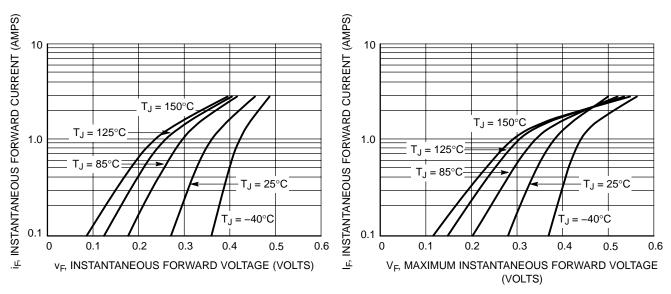
Figure 1. Typical Forward Voltage
