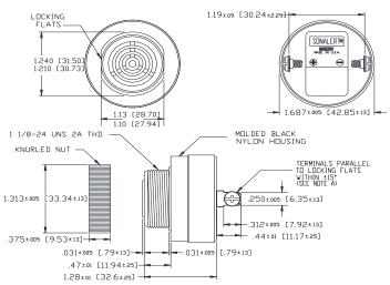
NOTE A: TERMINALS-032 BRASS TIN PLATED, TAPPED FOR #6-32 SCREW. TVD #6-32 NICKEL PLATED BRASS SCREWS INCLUDED. WILL ACCEPT 1/4\* QUICK CONNECT. NOTE B: MOUNTING- REMOVE BLACK PLASTIC NUT AND INSERT THREADED FRONT THROUGH 1.25' HOLE PUNCHED IN PANEL, IF DRIENTATION IS NEEDED, NOTE LOCKING FLATS ON DRAWING, SCREW NUT BACK ON. DO NOT OVERTIGHTEN.
