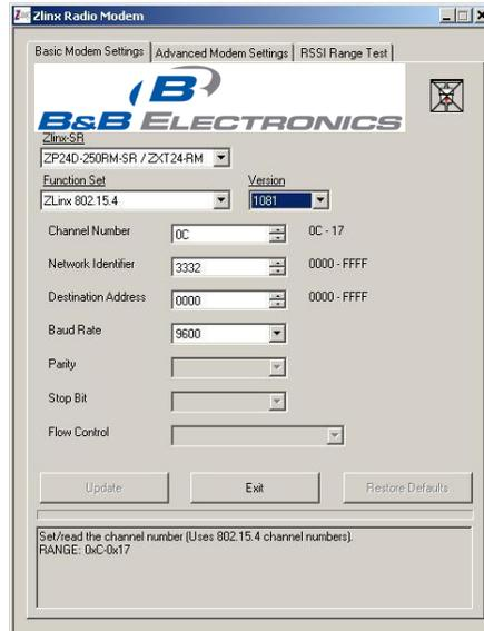
Figure 6-1 Radio Modem Basic Settings
