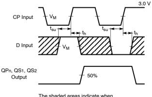
The shaded areas indicate when the input is permitted to change for predictable output performance.
