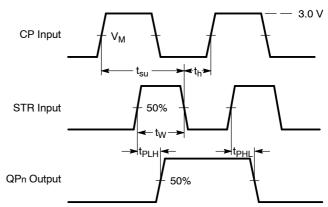
Figure 8. Waveforms showing the strobe (STR) to output (QPn) propagation delays, the strobe pulse width, the clock set-up and hold times for the strobe input.
